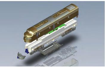
Step 3: Remove plow and coupler. The plow is held in place by two pin. Pull straight out to remove.
