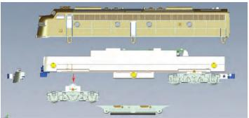
Step 6: With the chassis separated, remove the front truck.
