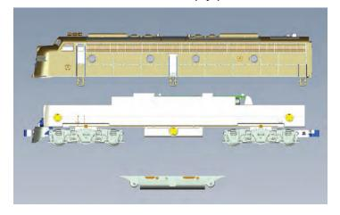
Step 2: Remove the fuel tank. The tank is pressure fit on. Pull down to remove.
