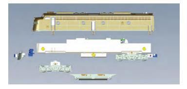
Step 7: Optional step - remove pilot mount (shown in blue). This is not necessary can be left in place.
