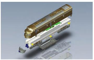
Step 4: Loose the three screws that hold the chassis in place. Keep the screws in place.
