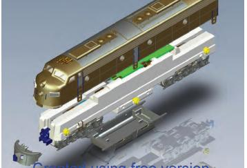
Step 5: Slightly sererate the split frame. There is no need to sererate completely. The goal is to unclamp the trucks from the chassis.
