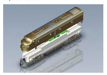
Step 1: Remove the shell. Inserting a small flat head screwdrive between the rear of the shell and chassis and prying up will make shell removal much easier. The shell is simply pressure fit on.
