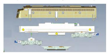
Step 8: Instal new truck with truck mounted couplers.
